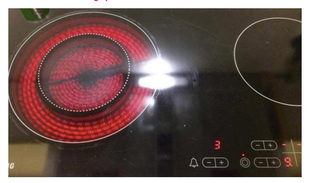
On the two larger rings there is an option to use two rings instead of one (for boiling or frying for example)
